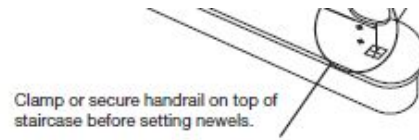
Fig-1 pre-assembled baluster
